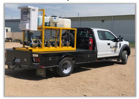
At Mountain Supply and Service we know that managing your cost is crucial. We are proud to offer a Chemical Injection Unit for use in coiled tubing or workover rig assisted snubbing applications for frac plug drillouts. Combined with our quality Completion Fluids, proper polymer hydration is ensured to provide a significantly enhanced drillout for the customer.
